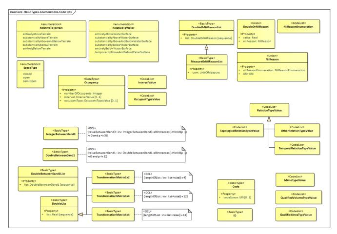
Figure 21. Basic Types, Enumerations, and Codelists from the CityGML Core module.
