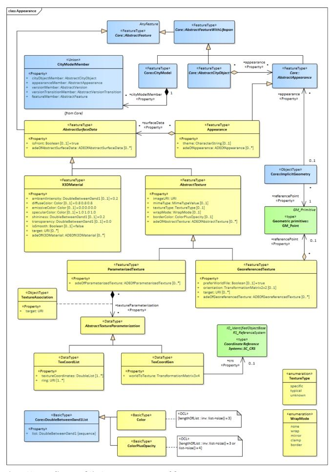
Figure 22. UML diagram of CityGML's Appearance model.
