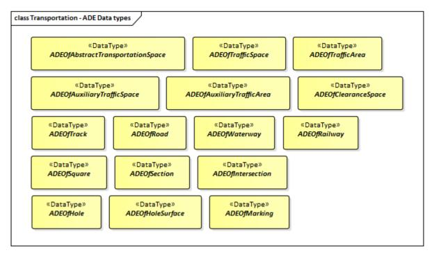
Figure 43. ADE classes of the CityGML Transportation module.
