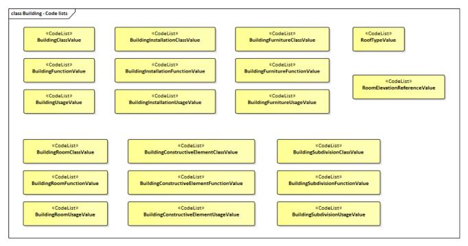
Figure 61. Codelists from the CityGML Building module.
