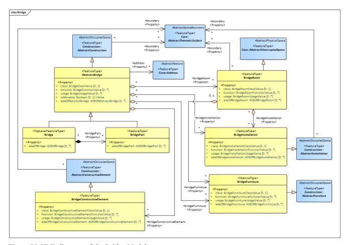
Figure 56. UML diagram of the Bridge Model.
