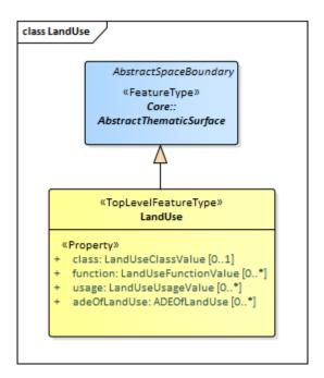
Figure 35. UML diagram of the Land Use Model.
