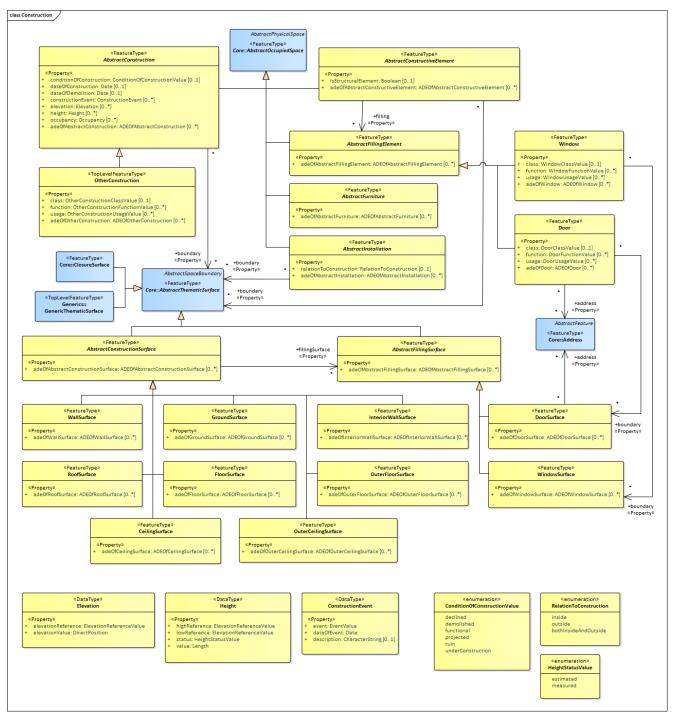
Figure 53. UML diagram of the Construction Model.
