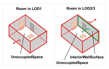
Figure 16. Representation of a room as UnoccupiedSpace in different LODs. The red boxes represent solids, the green area represents a surface. In addition, the normal vectors of the room solid (in red) and the wall surface (in green) are shown.
