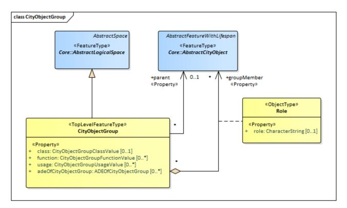
Figure 26. UML diagram of the City Object Group Model.
