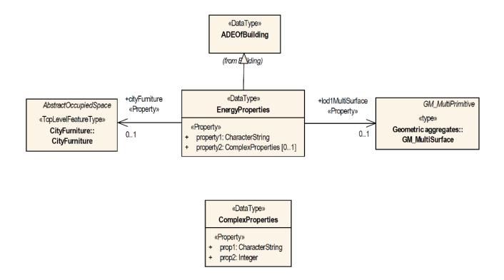
Figure 66. The CityGML feature type Building is augmented with additional ADE properties by defining the data type EnergyProperties as a subclass of the ADE data type ADEOfBuilding.
