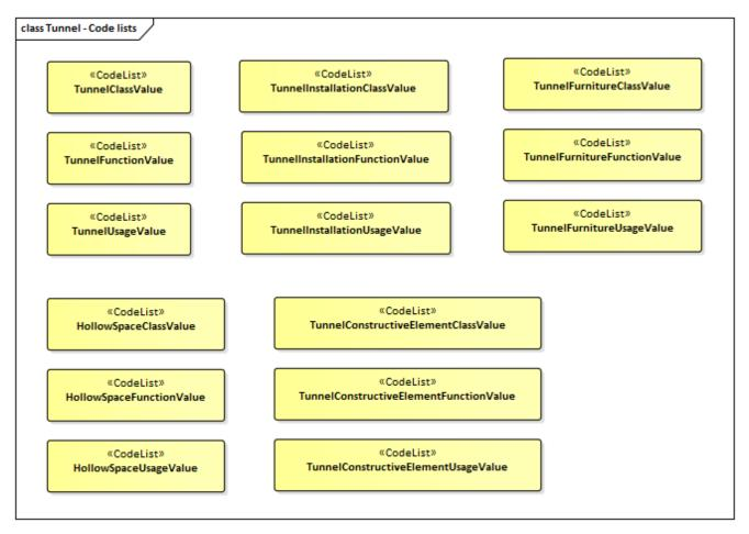
Figure 64. Codelists from the CityGML Tunnel module.
