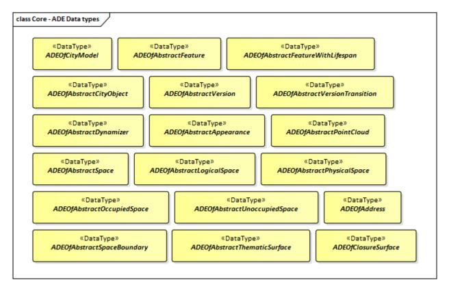
Figure 20. ADE classes of the CityGML Core module.
