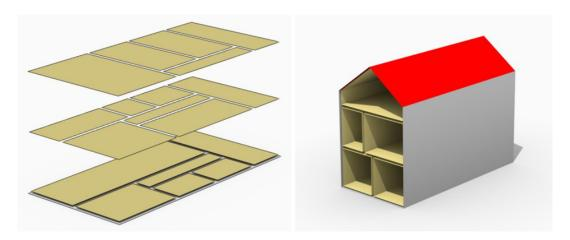
Figure 8. Floor plan representation (LOD0) of a building (left), combined LOD2 indoor and outdoor representation (right). Image adopted from Löwner et al. 2016.
