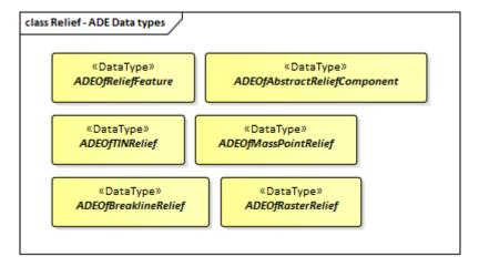
Figure 41. ADE classes of the CityGML Relief module.
