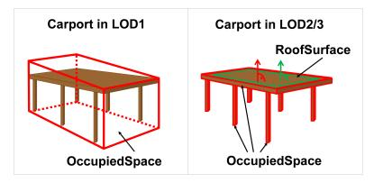
Figure 15. Representation of a carport as OccupiedSpace in different LODs. The red boxes represent solids, the green area represents a surface. In addition, the normal vectors of the roof solid (in red) and the roof surface (in green) are shown.
