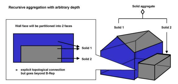
Figure 4. Recursive aggregation of objects and geometries in CityGML (graphic: IGG Uni Bonn).
