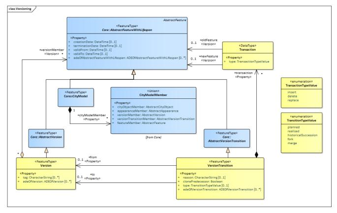
Figure 48. UML diagram of the Versioning Model.
