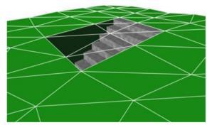
Figure 9. Closure surfaces to seal open structures. Passages are subsurface objects (left). The entrance is sealed by a virtual ClosureSurface feature, which is both part of the DTM and the subsurface object (right) (graphic: IGG Uni Bonn).
