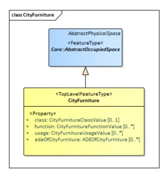
Figure 24. UML diagram of CityGML's City Furniture model.
