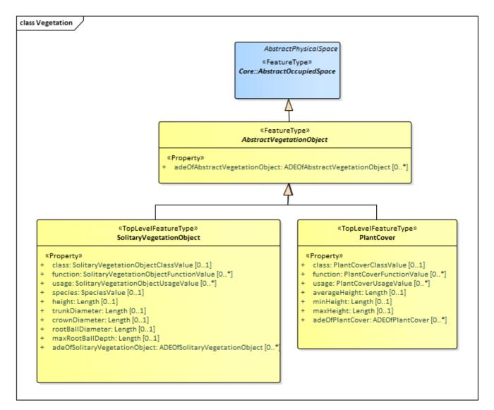
Figure 45. UML diagram of the Vegetation Model.
