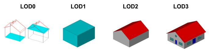
Figure 7. Representation of the same real-world building in the Levels of Detail 0-3.
