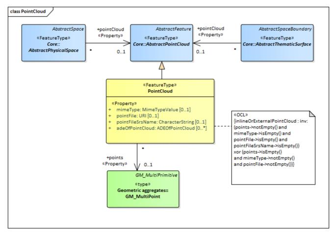
Figure 38. UML diagram of the Point Cloud Model.
