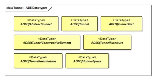
Figure 63. ADE classes of the CityGML Tunnel module.
