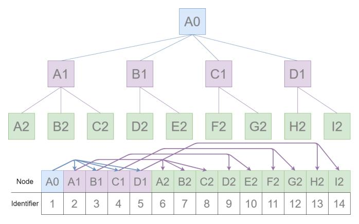
Example of breadth first ordering of nodes in a flat array. Children nodes are addressed by their index in the array.
