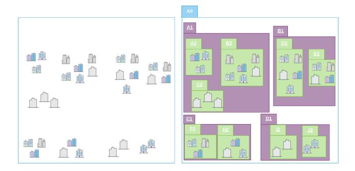
Schematic view of spatially distributed data and recursive grouping of nodes into a bounding volume hierarchy.
